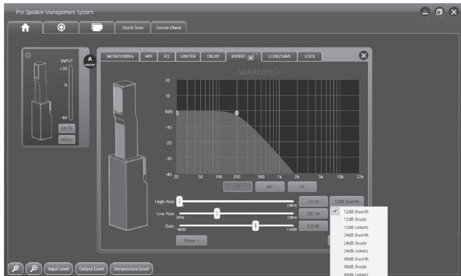
A crossover is used to divide the broadband signal into separate frequency bands. This allows each driver in a speaker system to be operated within its optimal frequency range. Using active crossover increase the efficiency of each driver but also of the amplifier by lowering the intermediation distortion.
